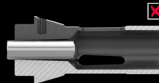
Visualization of a punctual ring clamping in the front area of the clamping surface
