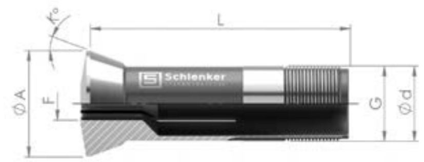
d Shaft-Ø A Head-Ø L Total length K Taper angle G Thread F Shape
