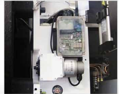
■ Absolute Encoder ATC System < NXV1680B is exclusive >
