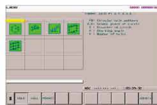
RECTANGULAR HOLE PATTERN (G120 P4) Function
